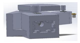
**Fig. 2.** Joint with Added Sensor and Motor
