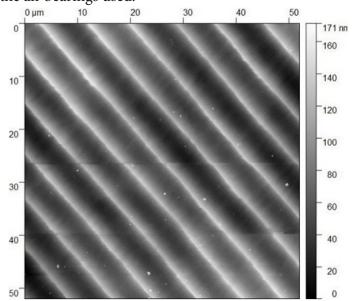
Fig. 4. AFM scan of copper part (500 rpm, 6 μm FPR).
