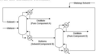
**Fig. 2** General extractive distillation process flow diagram.
