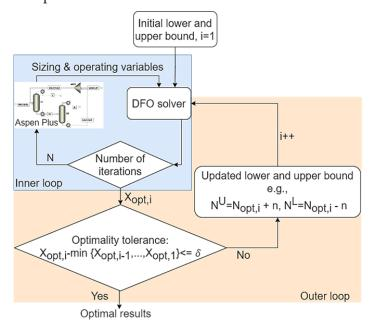
**Fig. 4** Derivative free optimization structure.
