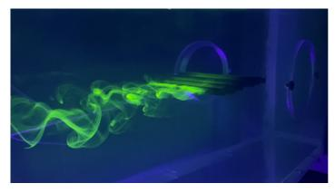
**Fig. 2** Water tunnel flow visualization (flow direction from right to left).
