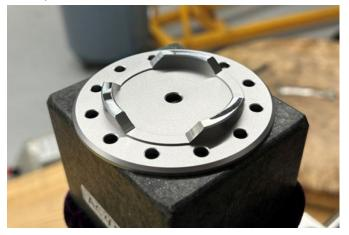
**Fig. 2.** The quasi-kinematic coupling used to eliminate inefficient workholding practices
