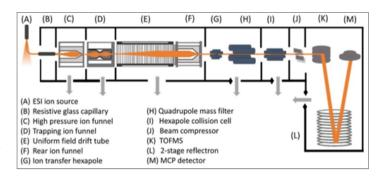
**Figure 2.** Schematic illustration of the Agilent 6560 Ion Mobility- Quadrupole Time of Flight- Mass Spectrometry instrument.
