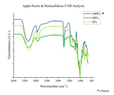
Fig. 1. FTIR Spectra of Apple Pectin Composite Films
