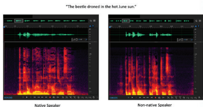
Fig. 1 Spectrograms show a native speaker of English (unaccented) and a non-native speaker of English (accented) saying “The beetle droned in the hot June sun.”
