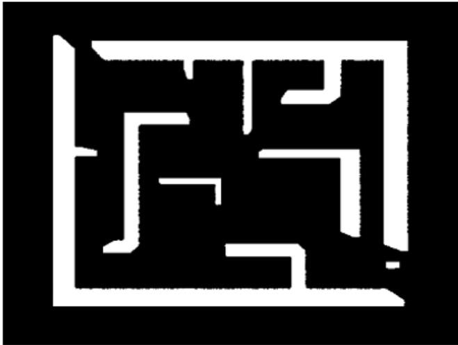
Fig. 2. Example of a region of interest mask output generated by this project's UGV localization program.
