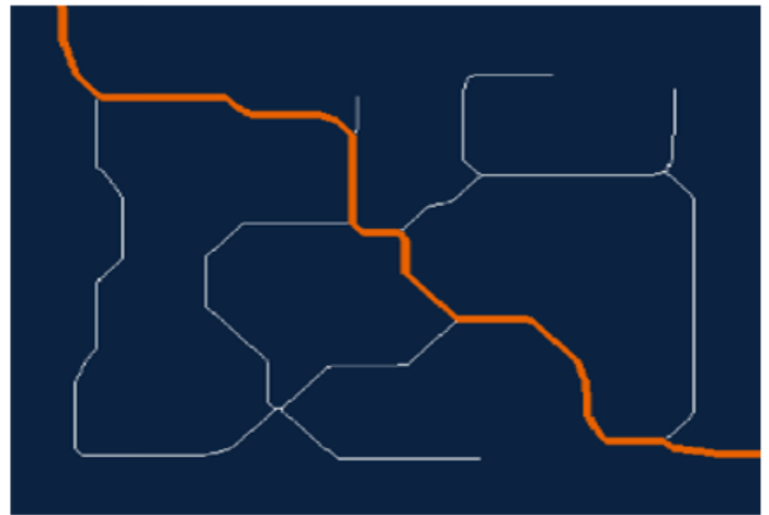
Fig. 4. Example of the shortest path output generated by the UGV's path planning program.
