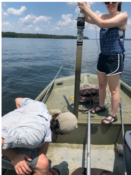
Fig. 1 Collection of a sediment core using a core barrel.
