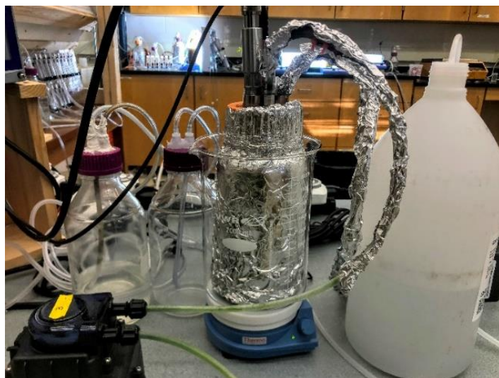
Fig. 1 PAO seeding reactor in operation.
