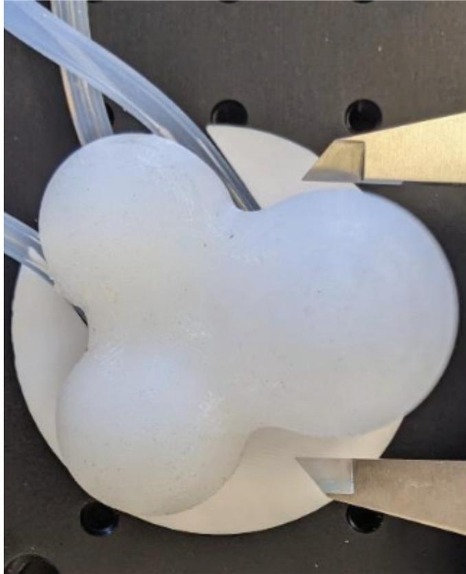
Figure 1. Final silicone mold inflating.
