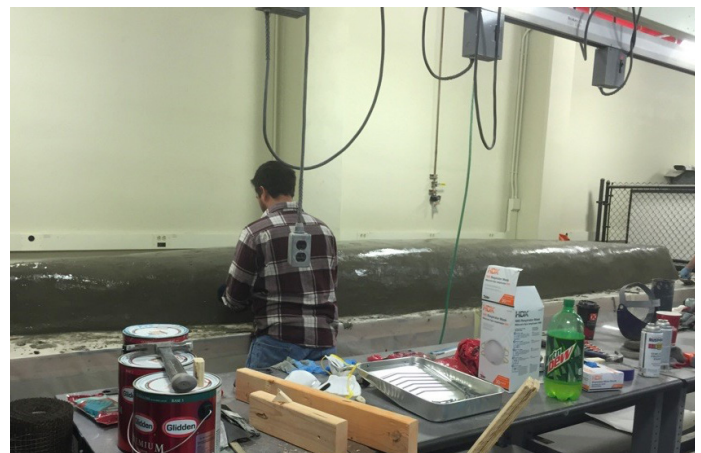
Photo: A member of the Auburn University chapter of the ASCE making the cast of the concrete canoe.
